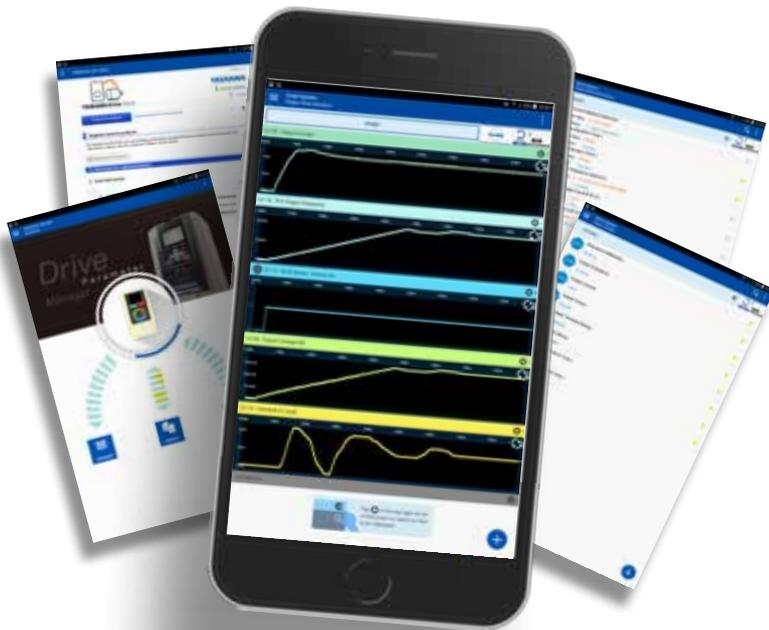
Mobile device connectivity is enabled using the built-in USB port (USB on-the-go) or via wireless communication with the Bluetooth® LCD keypad option.
